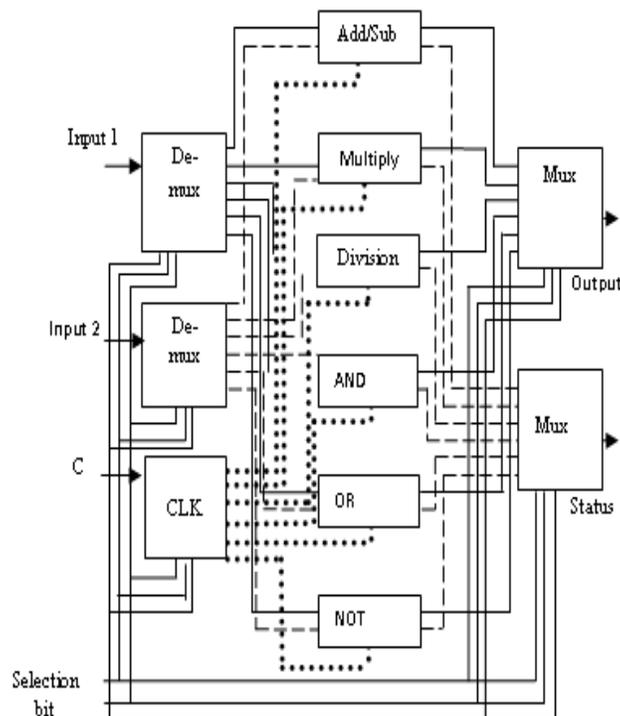
Figure 1: Top view of A.L.U. design
