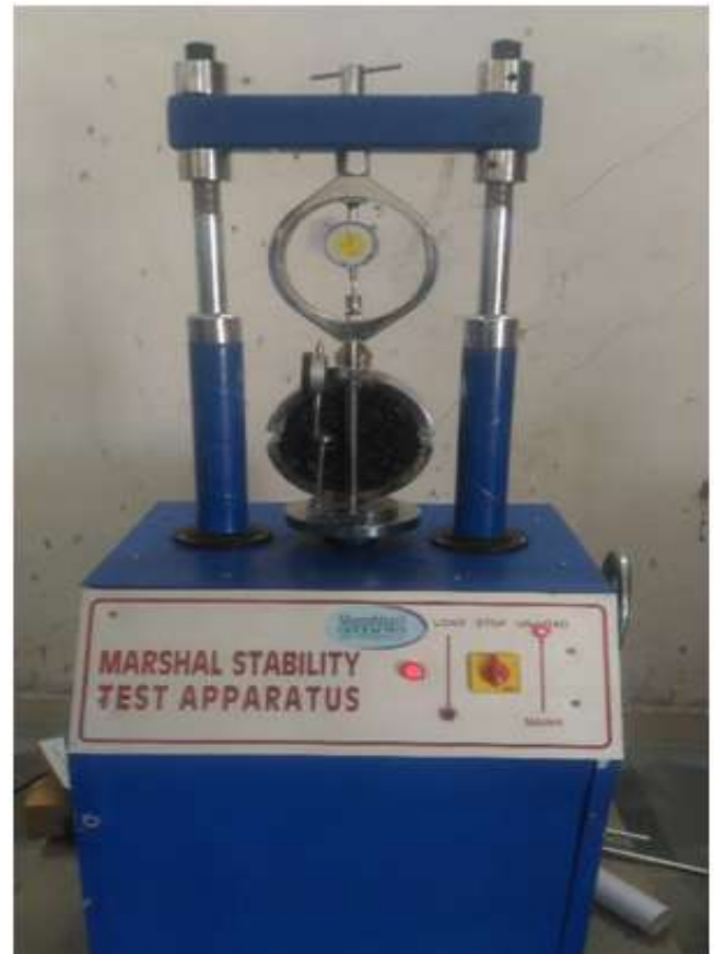
Figure 2.7: Marshal Stability Apparatus while performing experiment
