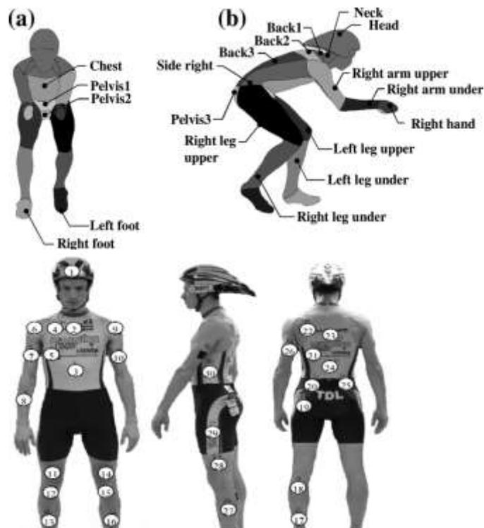
Fig (8): Locations of the pressure plates on the cyclist's surface (30 plates in total).
