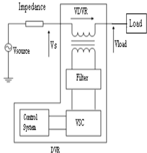
Figure 3: Block Diagram of Proposed Work
