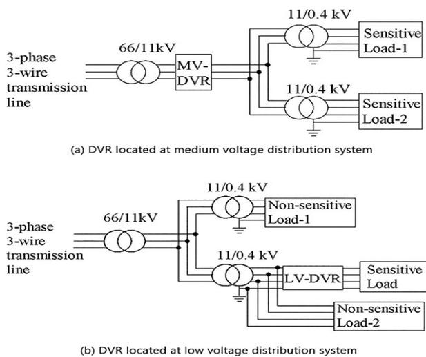
Figure 2: DVR topologies based on distribution line voltage levels
