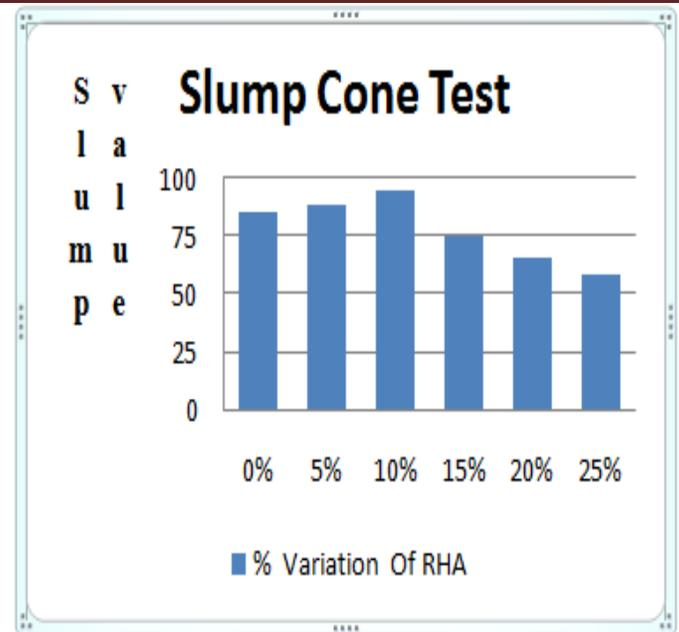
Workability of steel reinforced concrete mixes were tested by slum cone test. The result of that shown in fig. 1. The slump value shows gradual increase and decreased as the percentage of Rice Husk Ash (RHA) increases. From above graph degree of workability of most of the samples lies in between 50 to 90 mm that means the degree of workability is medium as per standard criteria
