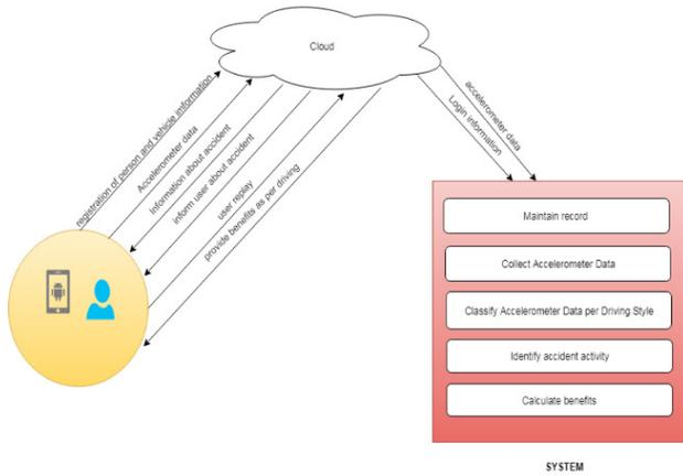
Figure 1: Block diagram
