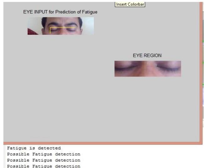
**Figure 6 :** Recognising if the eyes of the person are close then shows the Fatigue is detected
