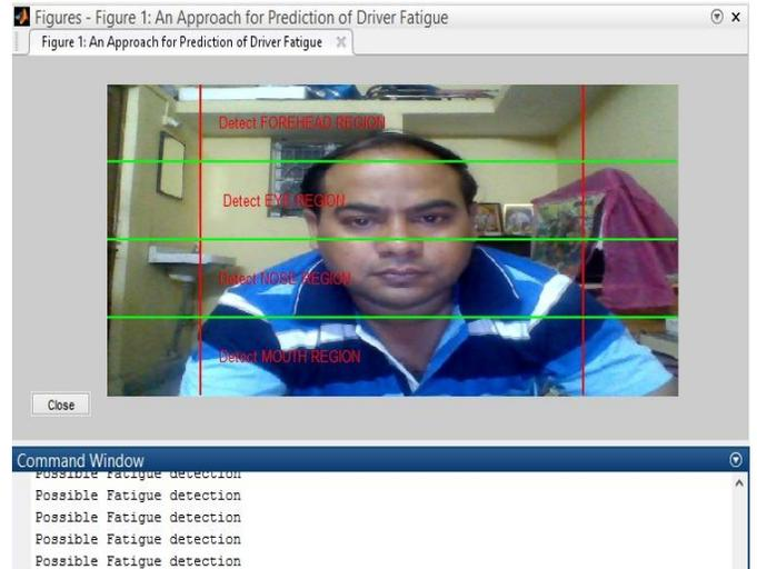
**Figure 5:** Fatigue Detection process initiated when the eyes of the person are open and the eye area are sliced means it shows the possibale Fatigue Detection.
